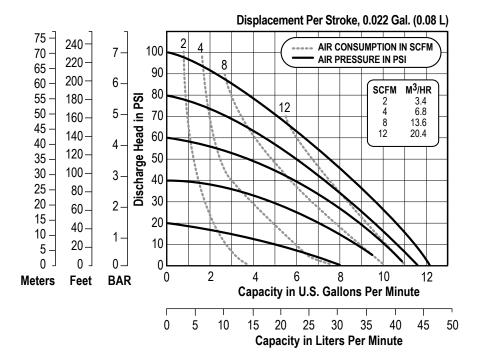
NOTE: Performance based on the following: PTFE fitted pump, flooded suction, water at ambient conditions. The use of other materials and varying hydraulic conditions may result in deviations in excess of 5%.
